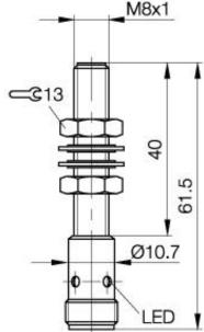
**Inductive Sensors** BES 516-377-S 4-C M8x1 x 61.5 normally-closed **Sn=1,5mm** shielded
